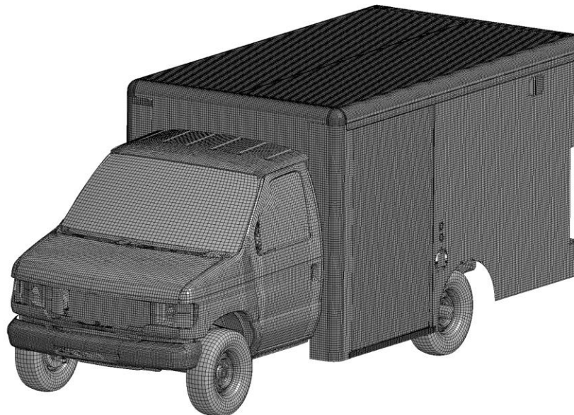
Figure 2. LS-Dyna Model of Production Ambulance
